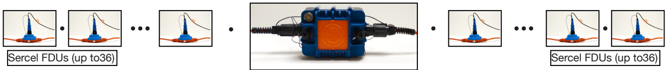
Figure 2: The layout of one Autonomous Recording Node with 72 FDUs
